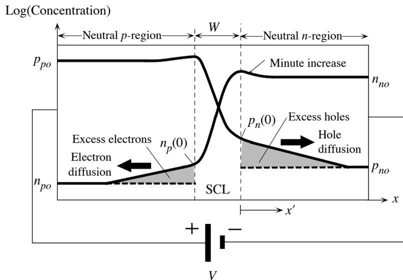
Forward biased  $pn$  junction and the injection of minority carriers. Carrier concentration profiles across the device under forward bias. Note: SCL = space charge layer and  $W$  = width of the SCL with forward bias. Other symbols have their usual meanings.
