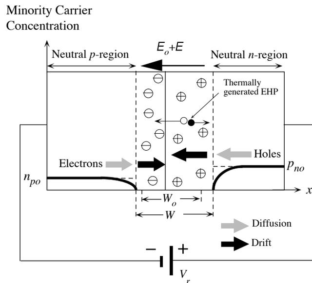
Reverse biased pn junction. Minority carrier concentration profiles and the origin of the reverse current. Note: EHP = electron-hole pair, SCL = space charge layer,  $\vec{E}$  = electric field,  $W$  = width of the SCL with reverse bias,  $V_r$  = reverse bias. Other symbols have their usual meanings. Subscript  $o$  refers to "no-bias" condition.
