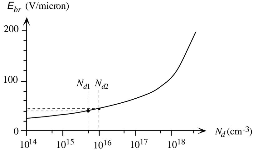
The breakdown field,  $E_{br}$ , in the depletion layer for the onset of reverse breakdown vs. doping concentration,  $N_d$ , in the lightly doped region in a one-sided ( $p^+n$  or  $pn^+$ ) abrupt  $pn$  junction. Avalanche and tunneling mechanisms are separated by the dashed line (data extracted from M. Sze and G. Gibbons, Solid. State. Electronics, **9**, 831 (1966))
