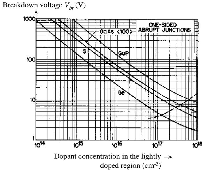
Avalanche breakdown voltage vs. dopant concentration in the lightly doped region of an abrupt  $pn$  junction. The dashed line indicates when tunneling breakdown begins to dominate as the dopant concentration increases further [Source: Figure 26 in *Physics of Semiconductor Devices, Second Edition*, S.M. Sze (John Wiley and Sons, New York, 1981) p.101]
